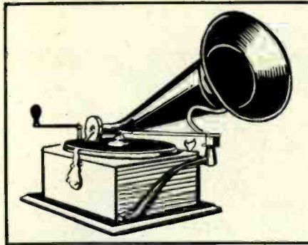
Fig. 5. The "Improved Gramophone" of the mid-nineties developed by Emile Berliner.
