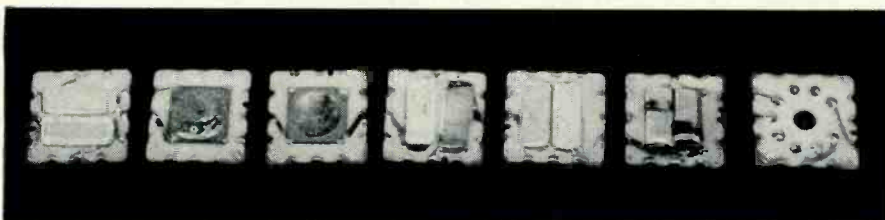
Fig. 4. Shown here are all the individual wafers contained in one typical module. The wafer on the right will hold a 9-pin miniature tube socket.
