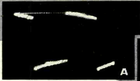
Fig. 6. Poor low-frequency response of the vertical amplifier of an oscilloscope results in the traces shown here when a square wave is used, see text.
