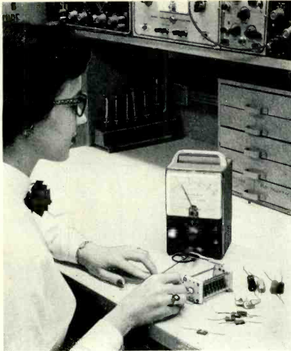
Barbara Szygielski, Heath Engineering secretary, demonstrates ease with which variable tuning capacitors may be measured with the direct-reading checker.
