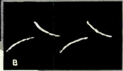
Fig. 6. Poor low-frequency response of the vertical amplifier of an oscilloscope results in the traces shown here when a square wave is used, see text.
