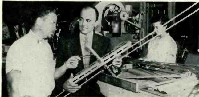
Fig. 2. A close-up look at the phasing element used in the "Wizard" TV antenna.
