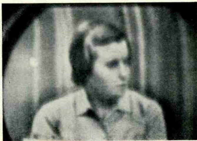
Fig. 6. Another case of left-hand hook combined with poor focus. This condition is often accompanied by instability.
